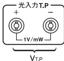
$$\text{光入力レベルP (dBm)} = 10 \log_{10} V_{T.P} (\text{V})$$
